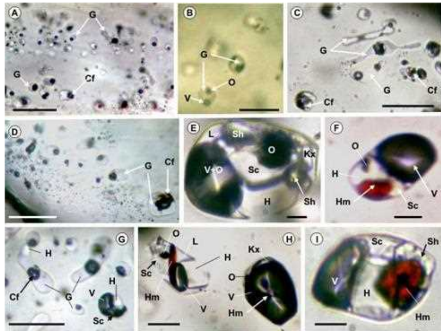
Fig. 5. Microphotographs showing several kind of silicate glass inclusions, vapor-rich and hydrous salt melt inclusions in quartz from Deva (A, C, D, E, F,G, I) and Rosia Poieni (B,H) porphyry copper systems. G-glass, Cf-saline fluid, H-halite, V-vapor, Sc- another salt daughter phase, Hm-hematite, Kx- unidentified solid phases, Sh- probable anhydrite, O-opaques - pyrite, magnetite, bornite etc; Scale bar = 20 microns.
