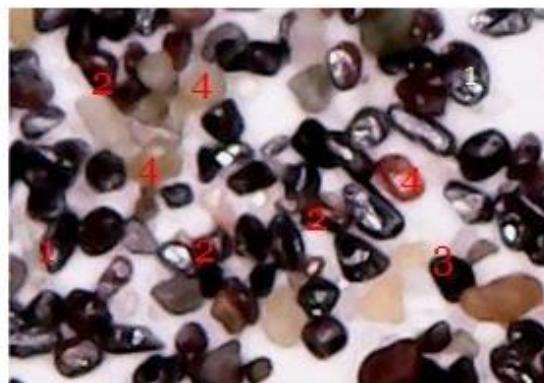
Photo 2: 1. zircon, 2. rutile, 3. hematite, 4. garnet; width of field: 500µm.
