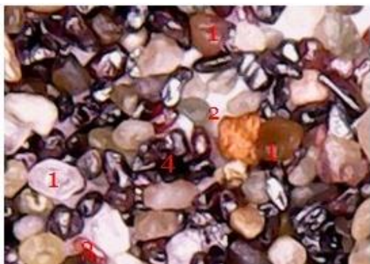
Photo 1: 1. garnet, 2. tourmaline, 3. rutile, 4. magnetite; width of field: 500µm.
