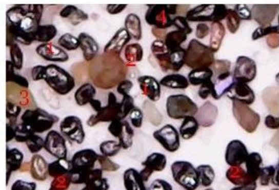
Photo 4: 1. garnet, 2. rutile, 3. zircon; width of field: 500µm.
