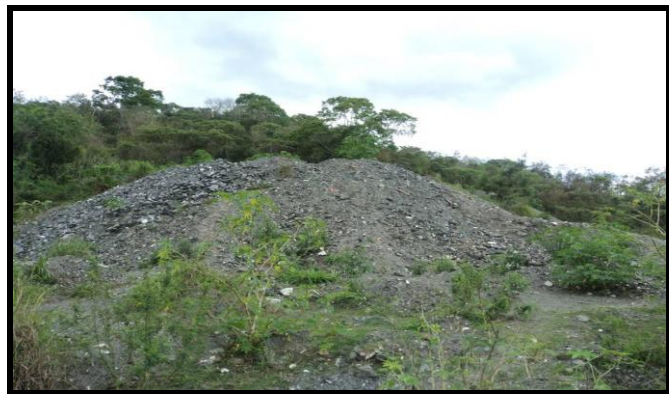
Fig. 2. Example of waste material used in the experiments. The material is composed of different schists, amphibolite and quartz veins.
