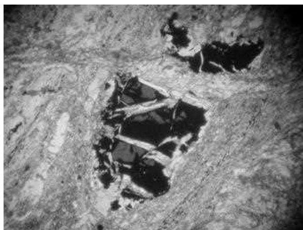
Foto 2. Divided chromite partially substituted by carbonates and phyllosilicates, Bradului Valley; x20 , NII
