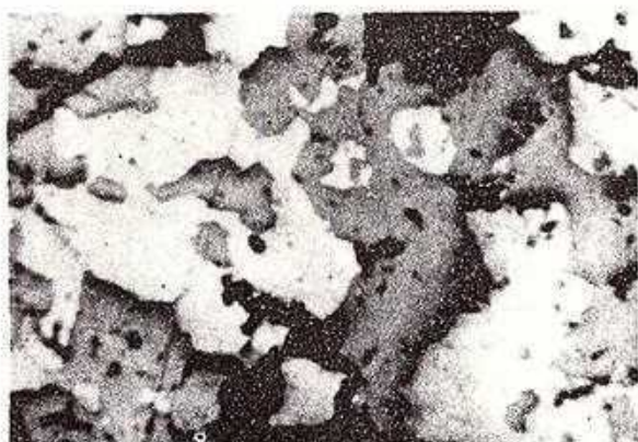
Fig. 3 - Sphalerite (grey) intergrown with galena (white); galena also occurs as subhedral inclusions, similar to the sphalerite ones in galena (see Fig. 1). RL, x 100.
