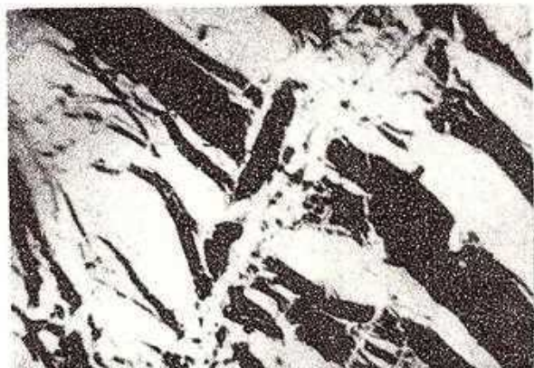
Fig. 1 – Parallel bands of pyrite (white) and silicates (black) crossed by pyrite veinlets, probably representing local regenerations. Reflected light (RL), x 150.
