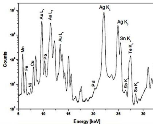
**Fig. 2.** The XRF surface analysis on an area of approx 1 mm by 1 mm of the investigated polished section from Roșia Montană. Maxima for Au, Ag, Sn, Te, Cu, Pb, Fe are visible in the spectrum (analyzed by Angela Vasilescu, from IFIN-HH Bucharest).
