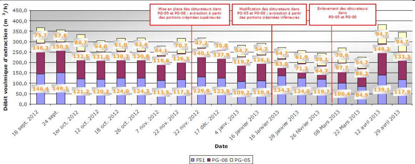
Evolution of the air extraction volume flow of each treatment well
