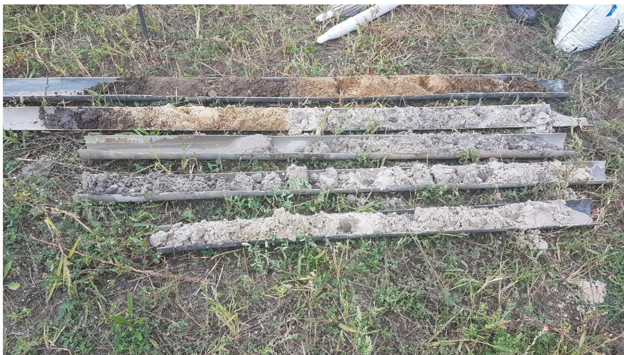
Drill core borehole (sonic drill)
