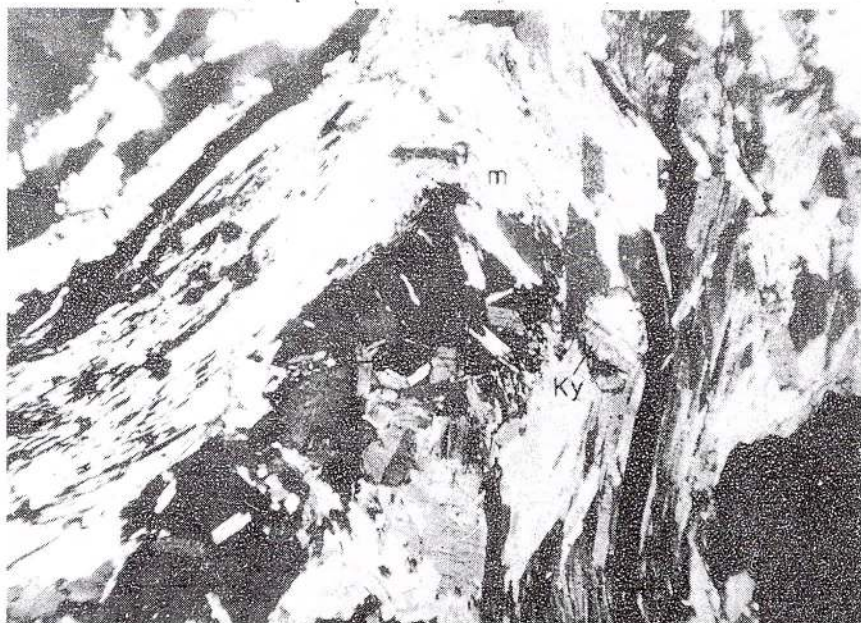
Fig. 1 - Rectilinear segments of micaceous minerals making up a fold. N+ ; 75X, m-micas, ky deformed kyanite crystal.
