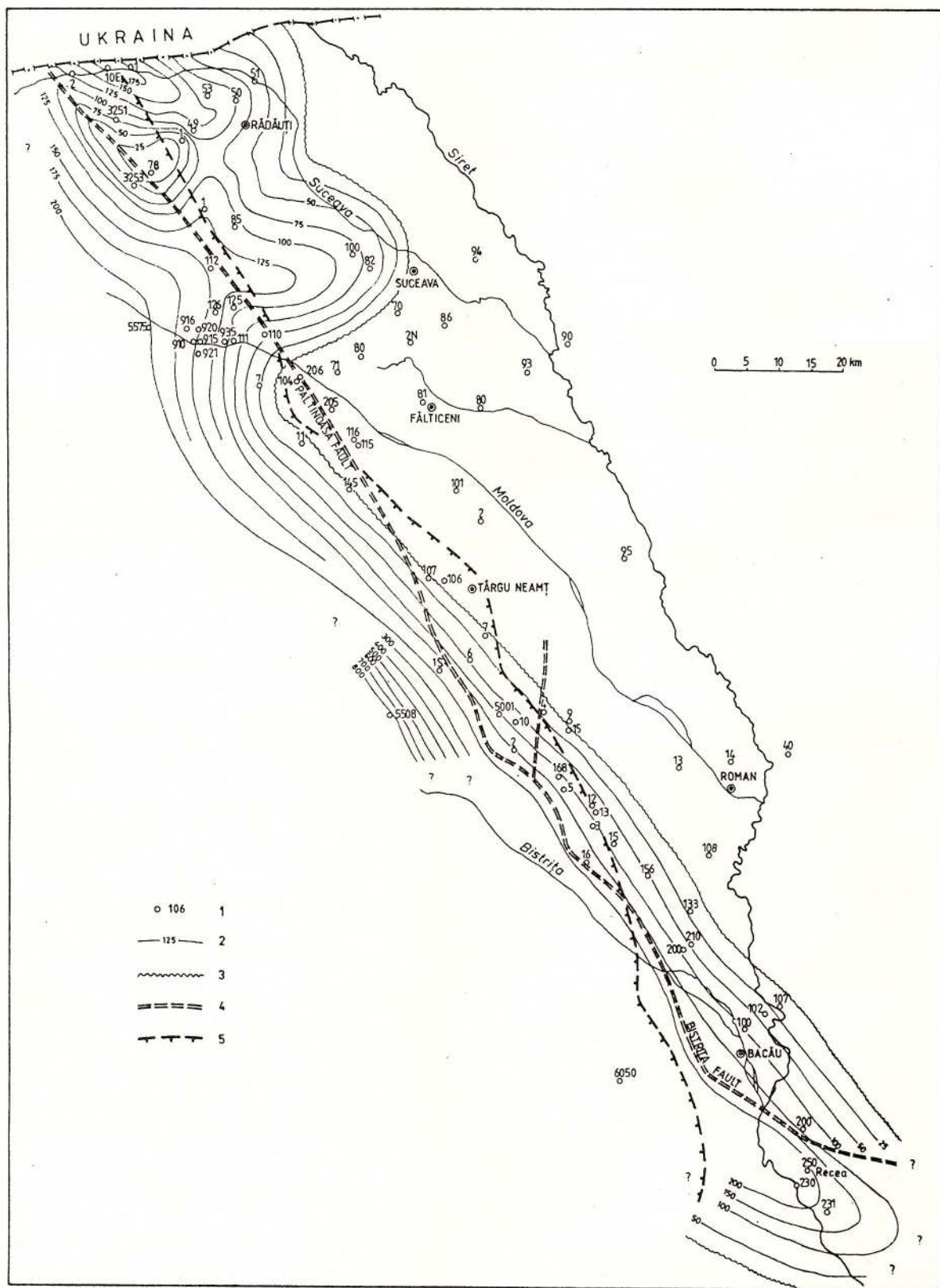
Fig. 1 – The western sector of the Eastern Carpathians Foreland map. Fragment with the thickness variations of the Upper Jurassic. 1, well with investigated samples; 2, isopach (equal thickness line); 3, shoreline; 4, fault; 5, overthrust line.
