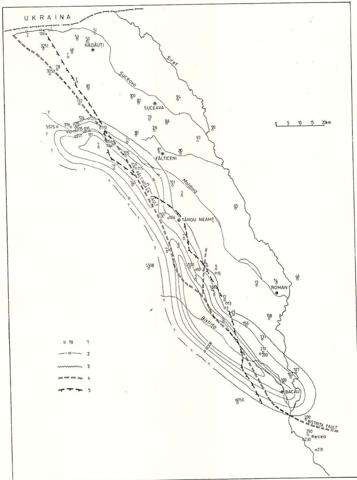
Fig. 10 - The western sector of the Eastern Carpathians Foreland map. Fragment with the thickness variations of the Danian-Paleocene. 1, well with investigated samples; 2, isopach (equal thickness line); 3, shoreline; 4, fault; 5, overthrust line.
