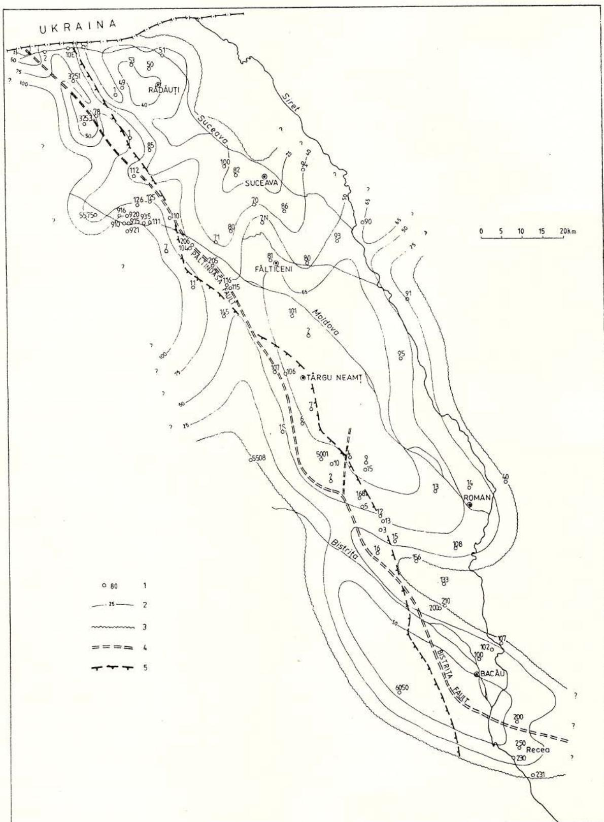
Fig. 6 -- The western sector of the Eastern Carpathians Foreland map. Fragment with the thickness variations of the Vraconian-Lower Cenomanian. 1, well with investigated samples; 2, isopach (equal thickness line); 3, shoreline; 4, fault; 5, overthrust line.
