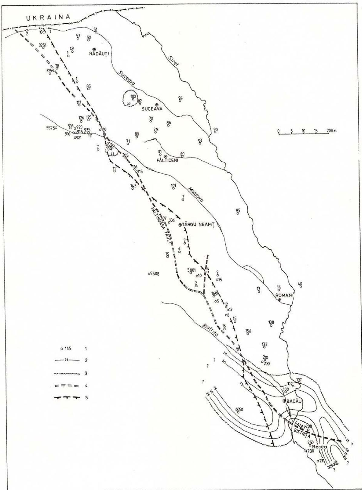
Fig. 4 – The western sector of the Eastern Carpathians Foreland map. Fragment with the thickness variations of the Aptian. 1, well with investigated samples; 2, isopach (equal thickness line); 3, shoreline; 4, fault; 5, overthrust line.
