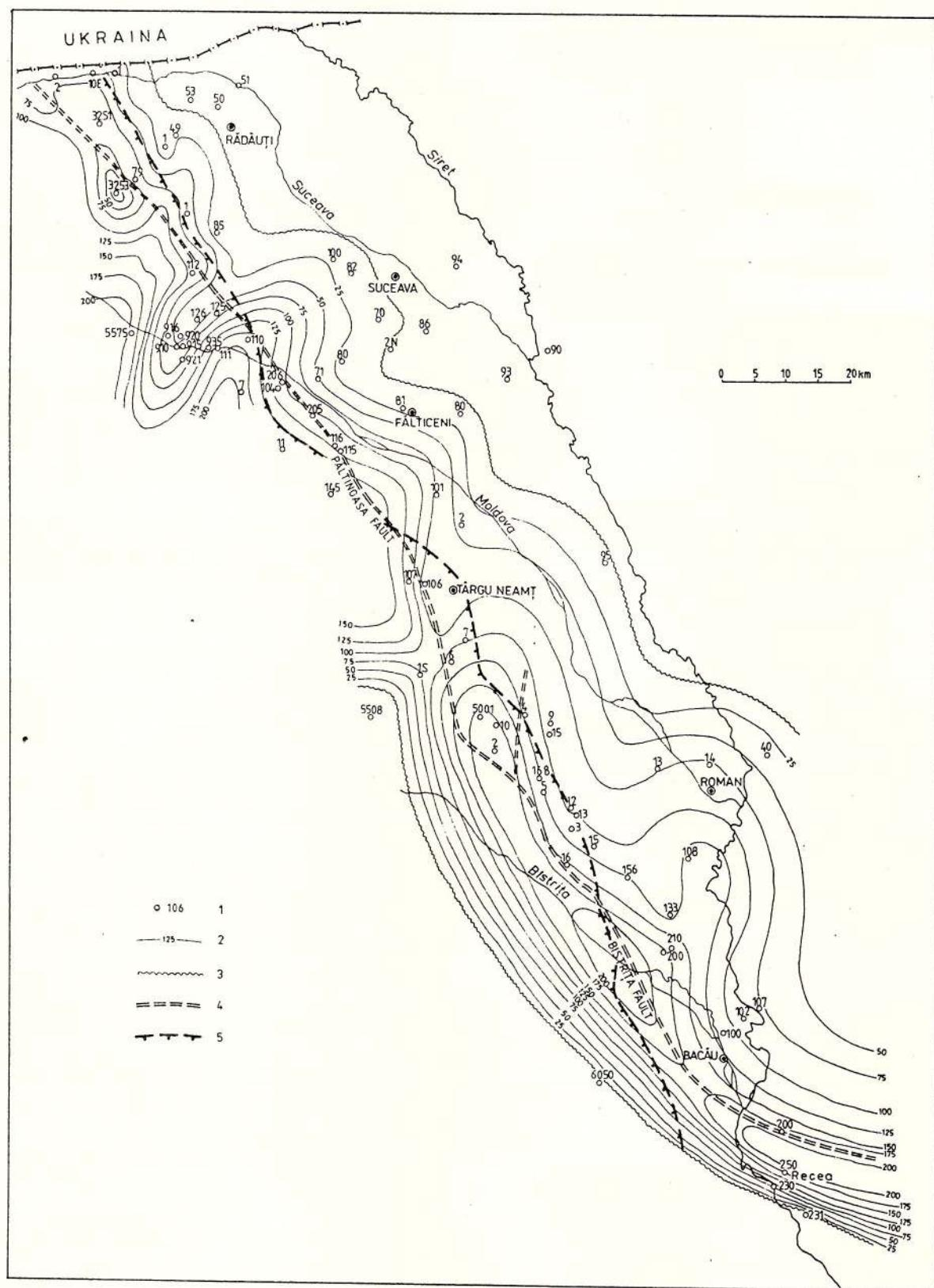
Fig. 9 – The western sector of the Eastern Carpathians Foreland map. Fragment with the thickness variations of the Upper Campanian. 1, well with investigated samples; 2, isopach (equal thickness line); 3, shoreline; 4, fault; 5, overthrust line.
