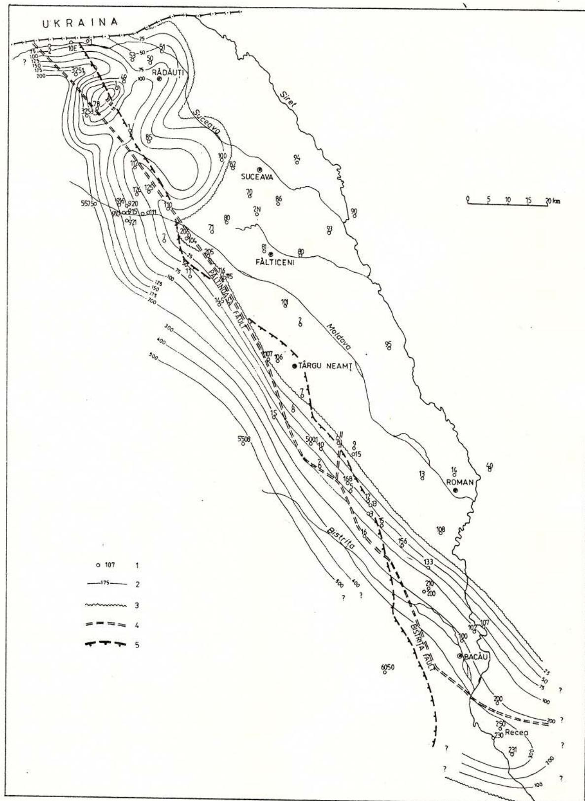
Fig. 2 – The western sector of the Eastern Carpathians Foreland map. Fragment with the thickness variations of the Berriasian-Lower Valanginian. 1, well with investigated samples; 2, isopach (equal thickness line); 3, shoreline; 4, fault; 5, overthrust line.
