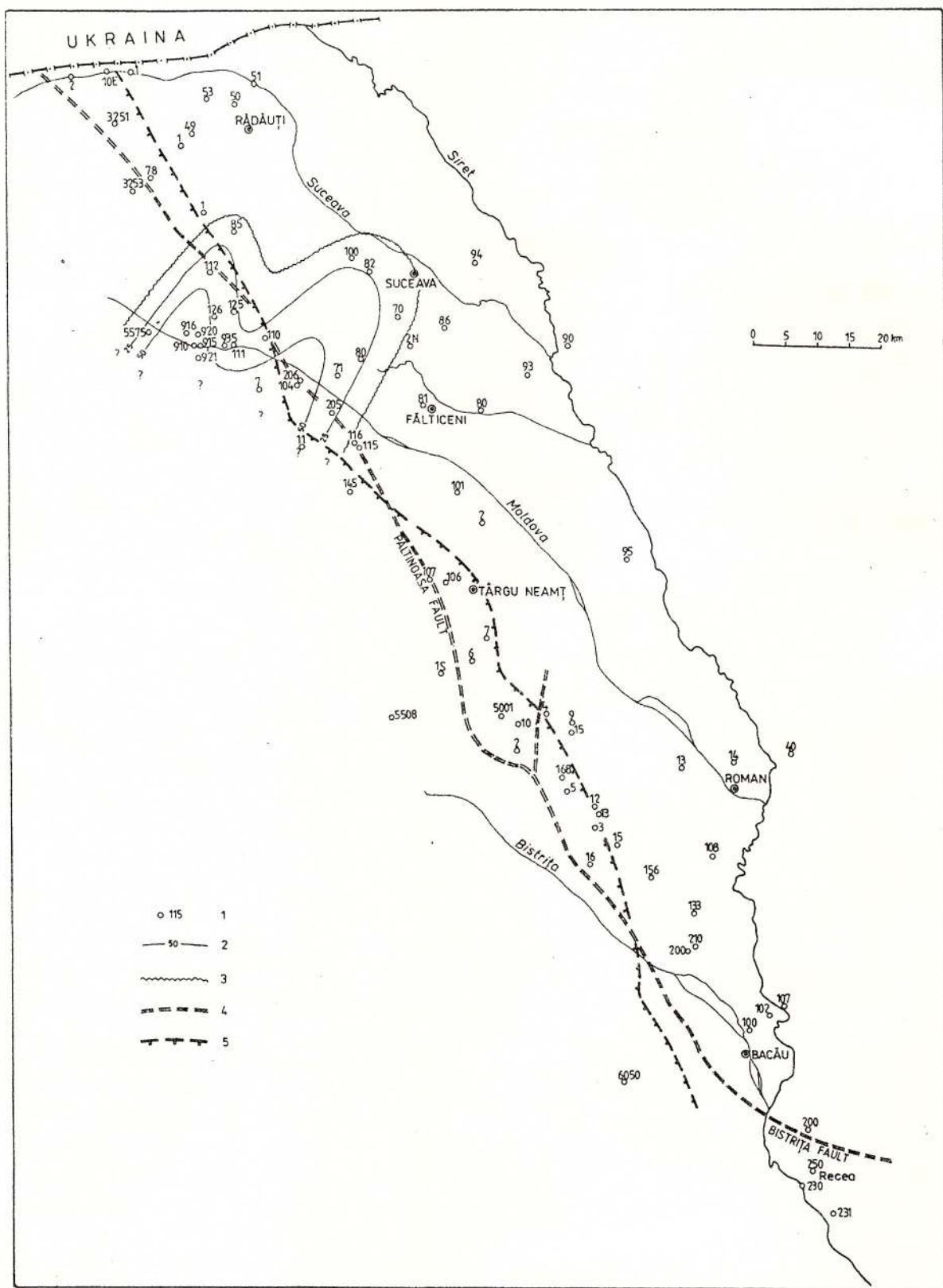
Fig. 5 – The western sector of the Eastern Carpathians Foreland map. Fragment with the thickness variations of the Upper Albian. 1, well with investigated samples; 2, isopach (equal thickness line); 3, shoreline; 4, fault; 5, overthrust line.
