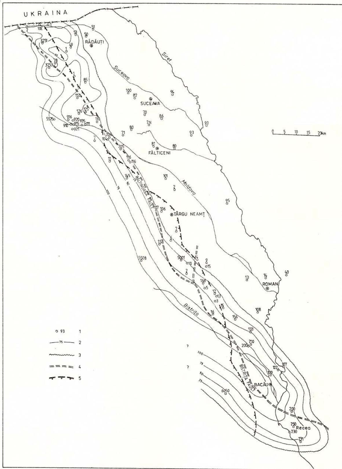
Fig. 3 – The western sector of the Eastern Carpathians Foreland map. Fragment with the thickness variations of the Upper Valanginian. 1, well with investigated samples; 2, isopach (equal thickness line); 3, shoreline; 4, fault; 5, overthrust line.
