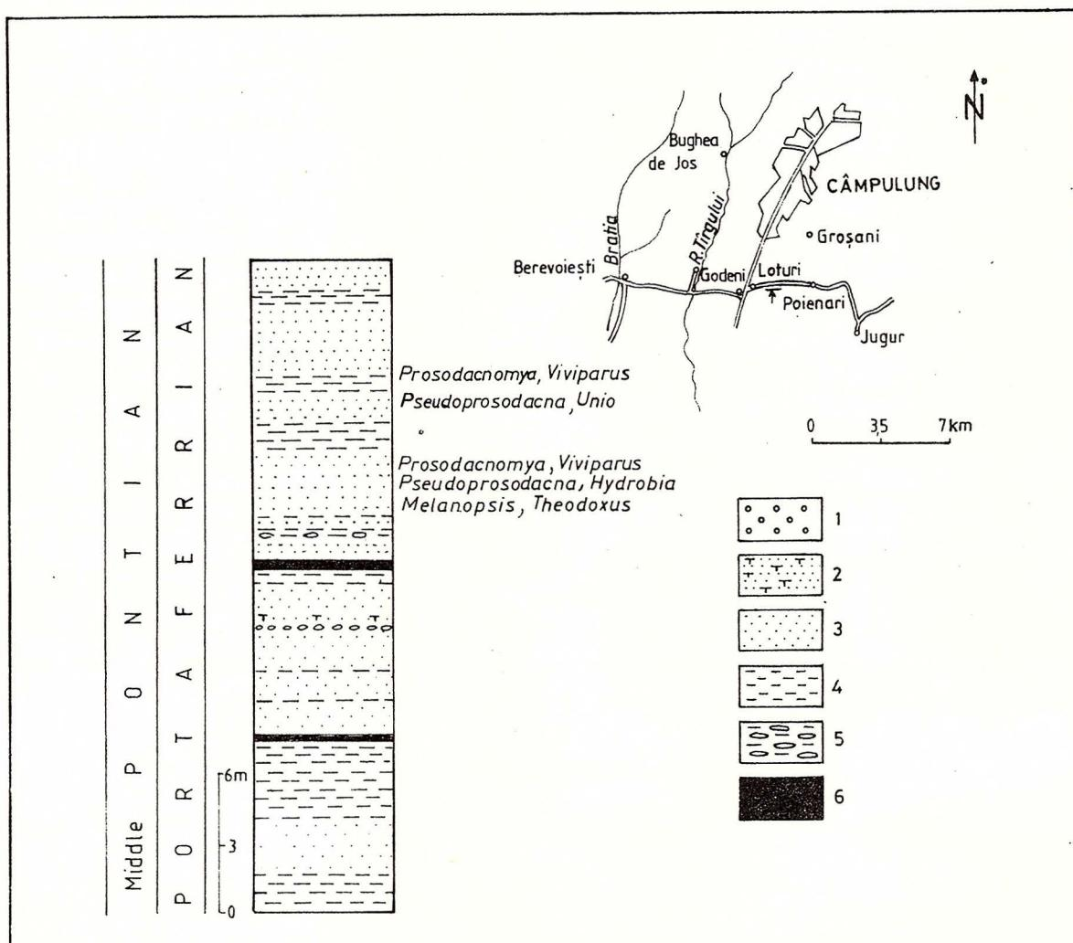
Fig. 2 – Stratigraphic column of the Middle Pontian (Portaferrian), Poienari village. 1, gravel; 2, slightly consolidated gritty sand; 3, sand; 4, clay; 5, clay with pebbles; 6, coal.
