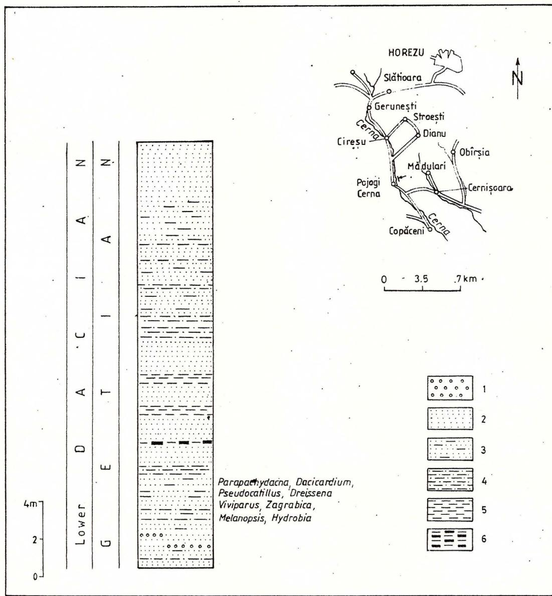
Fig. 9 - Stratigraphic column of the Lower Dacian (Getian) Pojogi village. 1, gravel; 2, sand; 3, clayey sand; 4, sandy clay; 5, clay; 6, coal clays.
