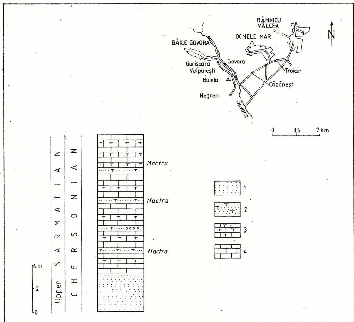
Fig. 7 – Stratigraphic column of the Chersonian, Buleta village. 1, sand; 2, slightly consolidated gritty sand; 3, calcareous sandstone; 4, limestone.
