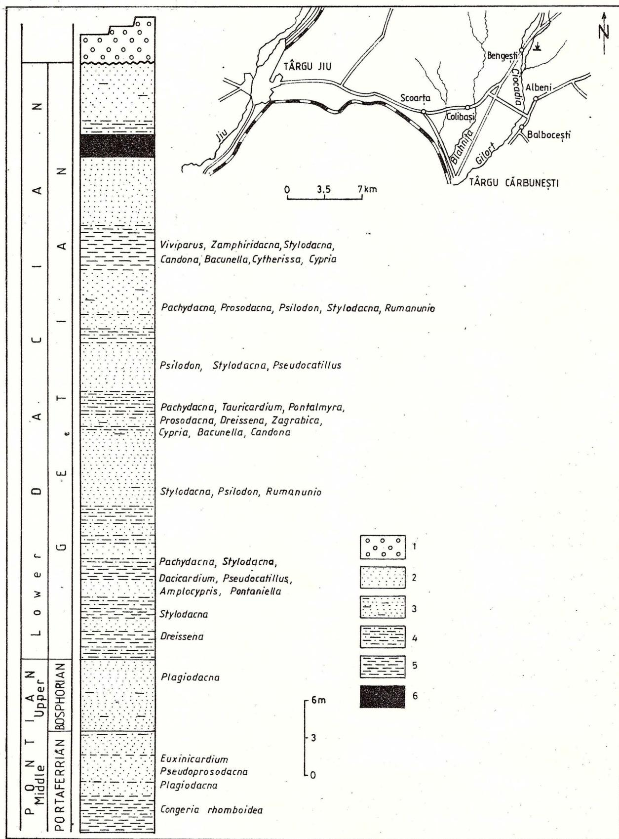
Fig. 10 – Stratigraphic column of the Pontian and of the Lower Dacian (Getian), Bengești village. 1, terrace gravel; 2, sand; 3, clayey sand; 4, sandy clay; 5, clay; 6, coal.
