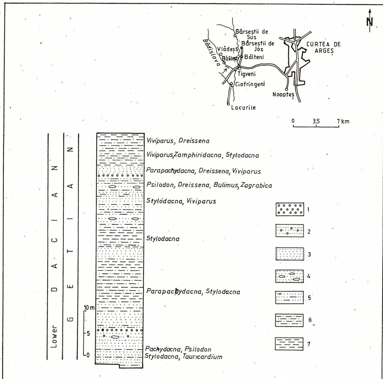
Fig. 4 – Stratigraphic column of the Lower Dacian (Getian) Bădislava Valley, Băilești village. 1, gravel; 2, sand with gravel; 3, sand; 4, sand with pebbles; 5, clayey sand; 6, sandy clay; 7, clay.
