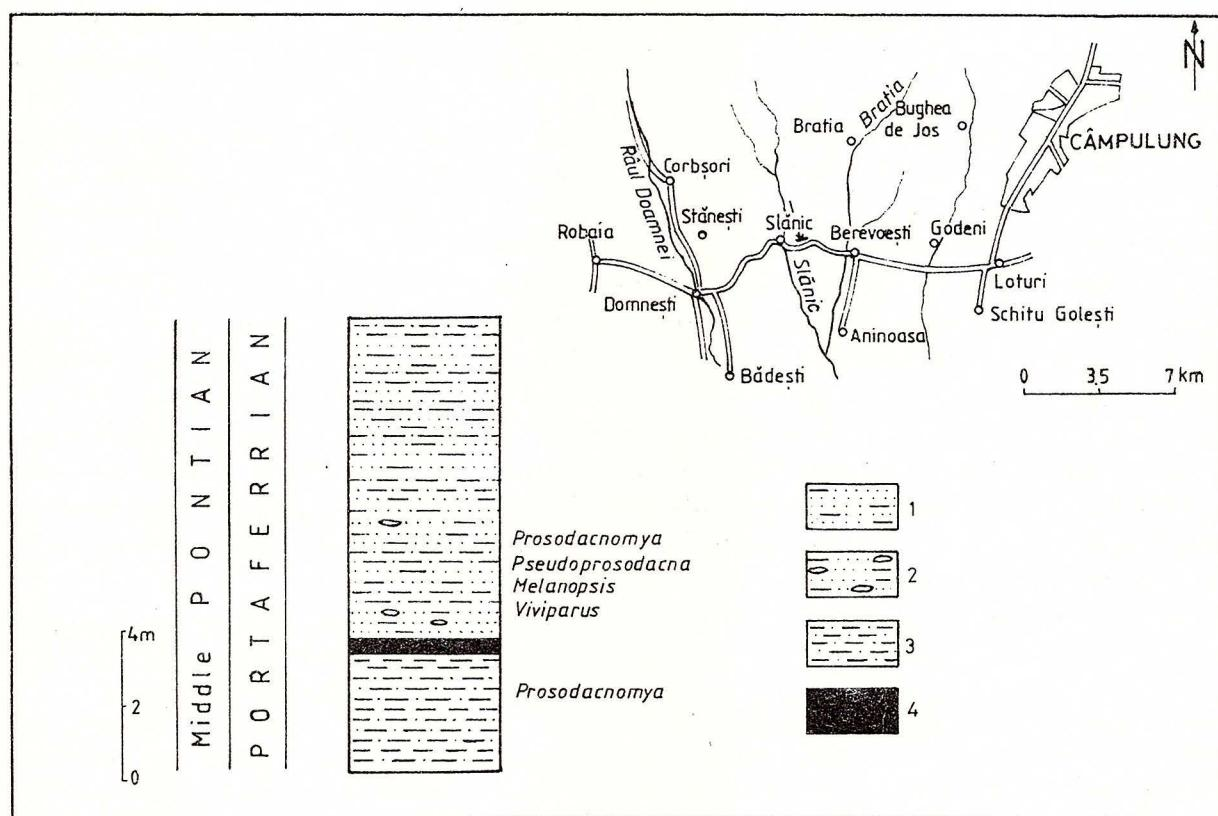
Fig. 3 - Stratigraphic column of the Middle Pontian (Portaferrian), between the Slănic village and the Bărevoești village. 1, clayey sand; 2, clayey sand with pebbles; 3, sandy clay; 4, coal.
