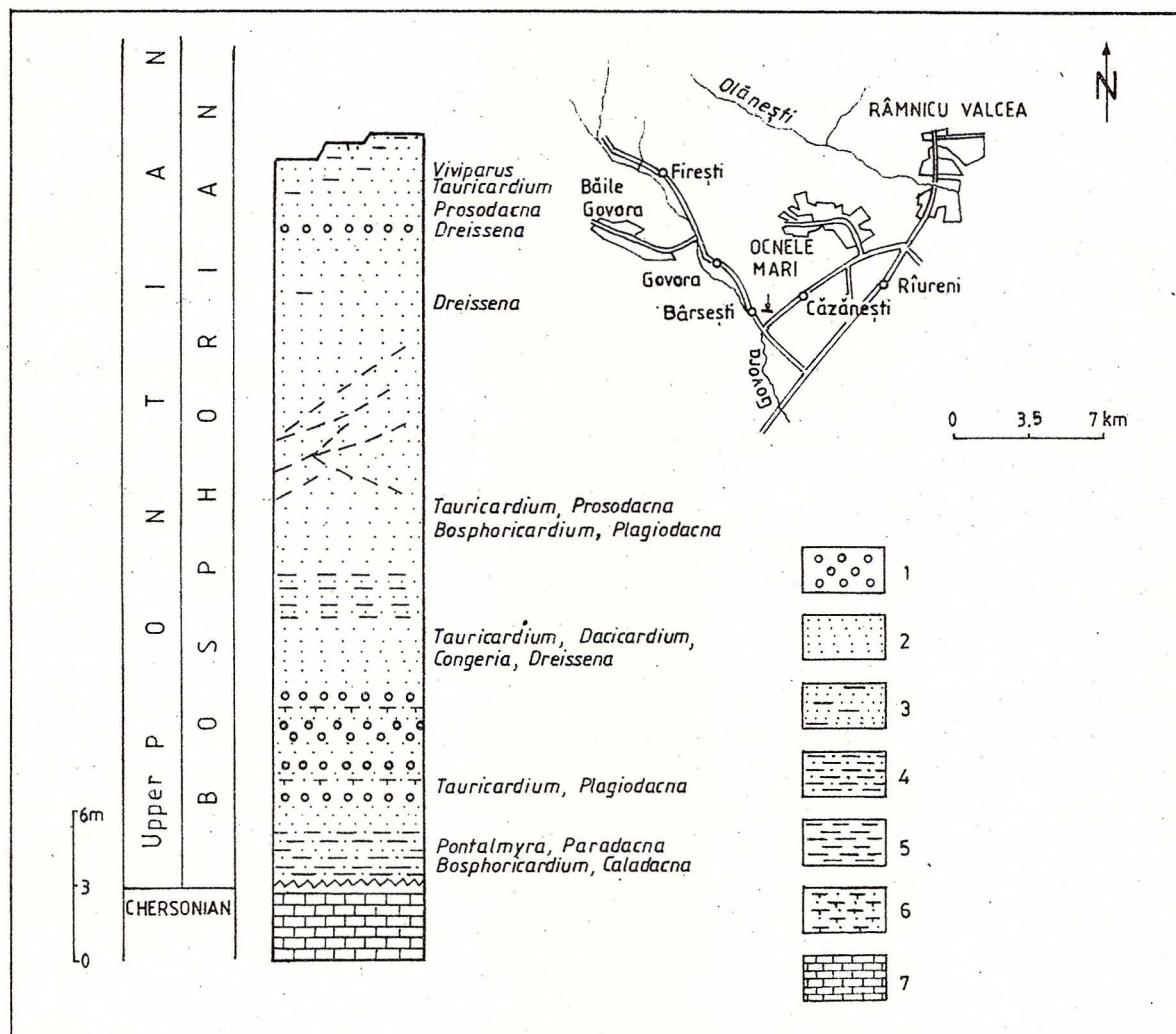
Fig. 6 - Stratigraphic column of the Upper Pontian (Bosphorian), Tuțurului Hill, Bârsești village. 1, gravel; 2, sand; 3, clayey sand, 4, sandy clay; 5, clay; 6, sandstone; 7, limestone.
