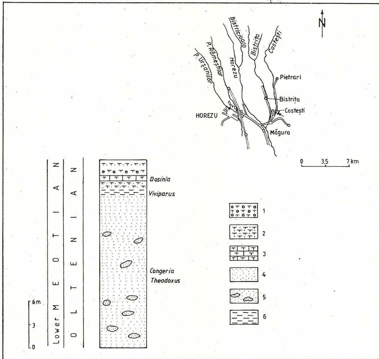
Fig. 8 – Stratigraphic column of the Lower Meotian (Oltenian), Costești village. 1, microconglomerate; 2, sandstone; 3, calcareous sandstone; 4, sand; 5, sand with concretions; 6, clay.
