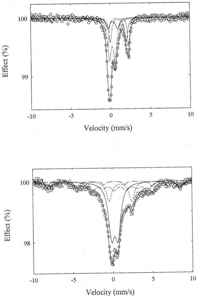
Fig. 3 – Mössbauer spectra for the sediment A3 at room (top) and the liquid helium temperature (bottom)
