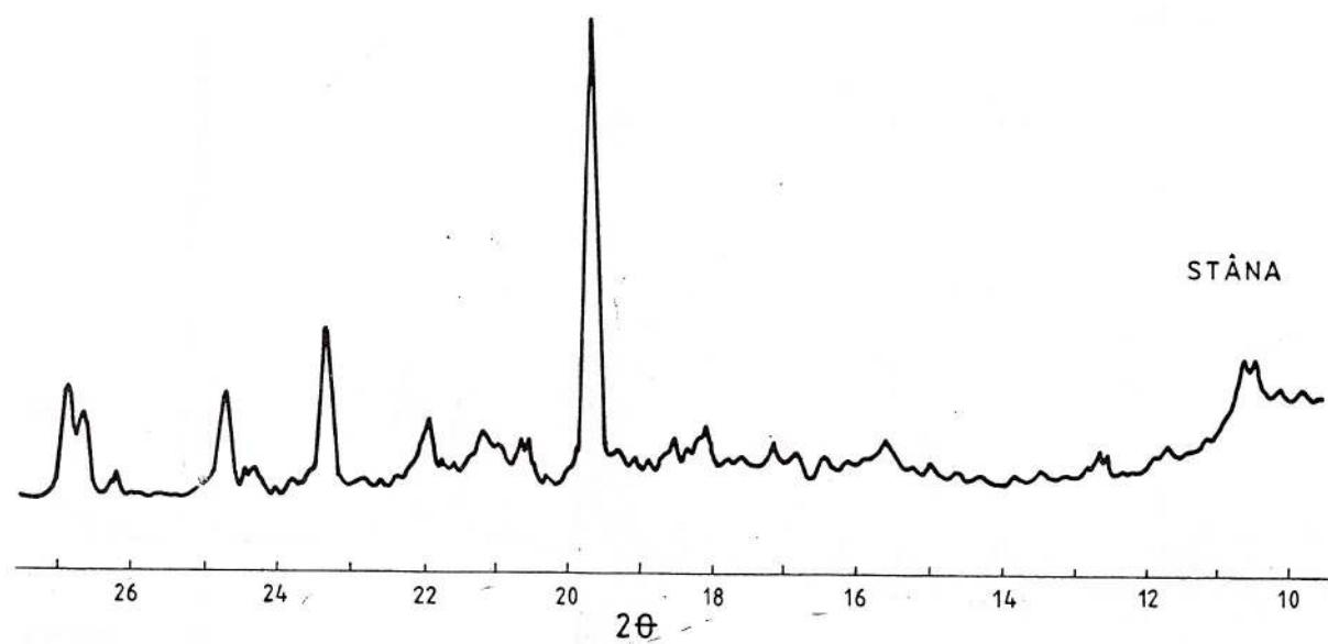
Fig. 5 – The X-ray analyses of clay intercalations from gypsiferous samples
