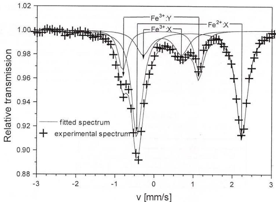
Fig. 3.1 - Mössbauer spectra of the sample 15c
