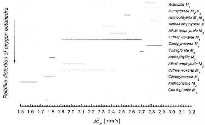
Fig. 2.7 - Quadrupole splitting versus octahedral distortion (Bancroft, 1973)
