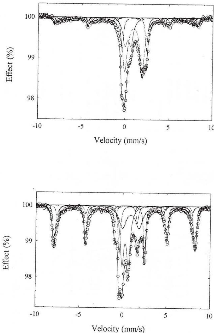
Fig. 2 – Mössbauer spectra of the sediments A1 (top) and A13 (bottom) magnetically split at room temperature
