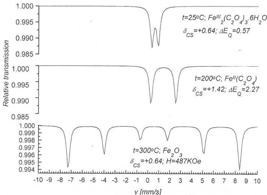
Fig. 2.12 - Mössbauer spectra for thermal decomposition of ferric oxalate
