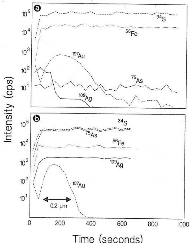
Fig. 6 – Depth profiles for two arsenopyrite grains (sample BBI-1), showing sub-microscopic inclusion of Au minerals.
