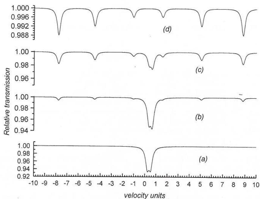
Fig. 2.14 - The Mössbauer spectra at room temperature for  $\alpha\text{-Fe}_2\text{O}_3$  for different particle size,
