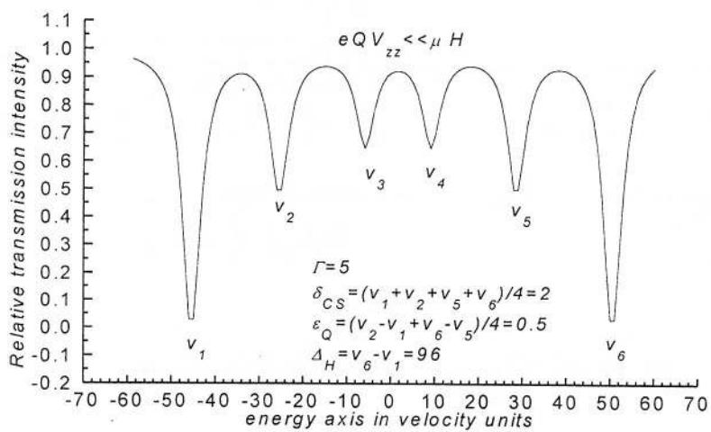
Fig. 1.7 - The spectra corresponding to the presence of hyperfine fields at Mössbauer isotope site
