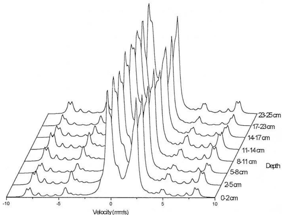
Fig. 8 - Envelopes obtained by the fitted Mössbauer spectra for the marine layers
