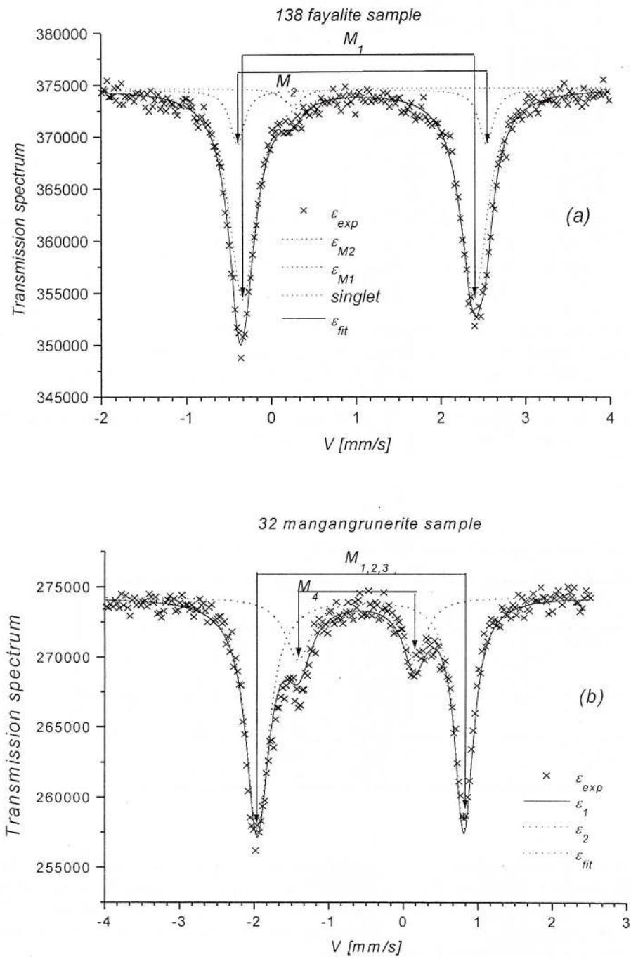
Fig. 3.2 - The spectra of 138 fayalite and of 32 mangangrunerite.
