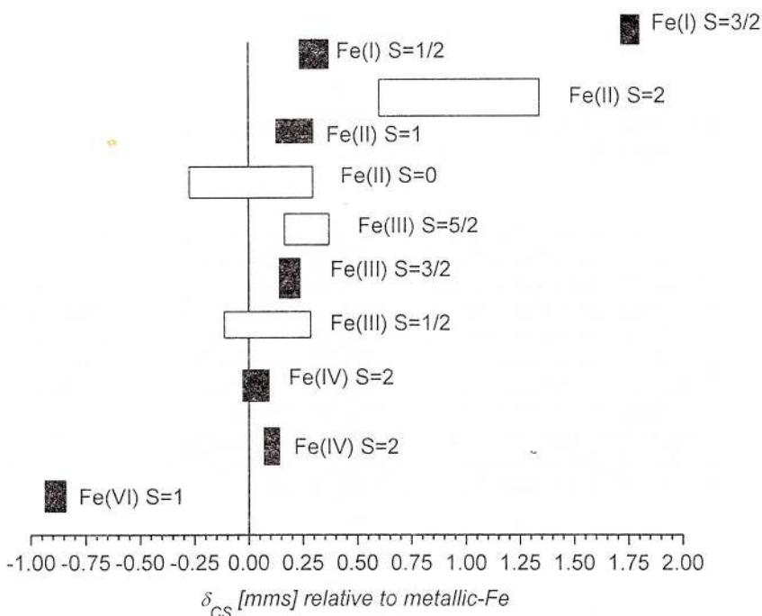
Fig. 2.1 - The central shift of iron compounds for different oxidation states and spin configurations
