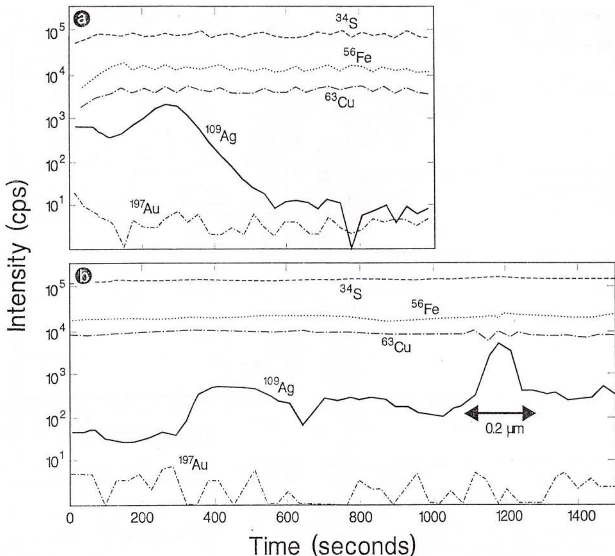
Fig. 4 – Depth profiles for two chalcopyrite grains (sample BB191), showing sub-microscopic inclusion of Ag minerals.
