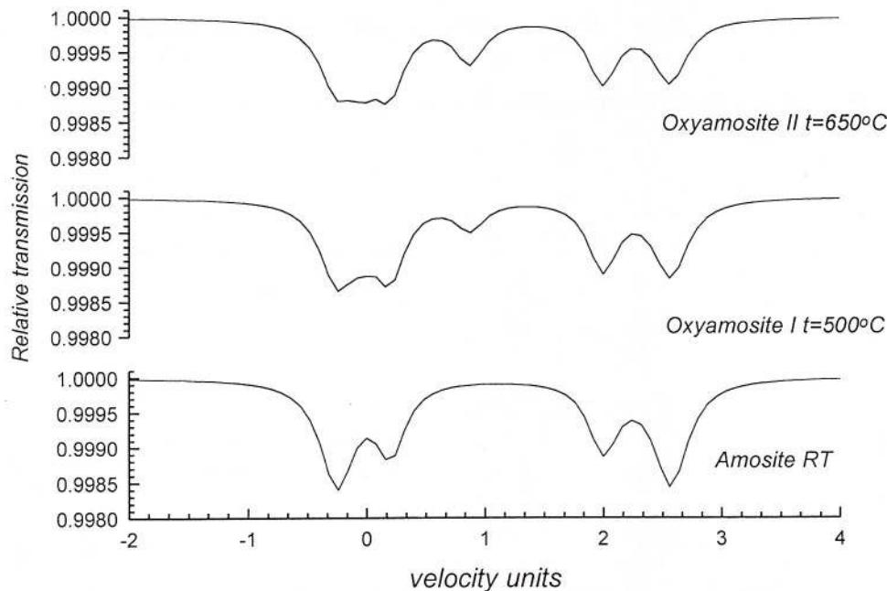
Fig. 2.11 - Mössbauer spectra of heated amosite
