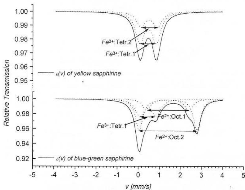
Fig. 2.4 - The Mössbauer spectra of two sapphires  $(\text{Mg},\text{Fe}^{2+})_2(\text{Al},\text{Fe}^{3+})_4\text{O}_6\text{SiO}_4$
