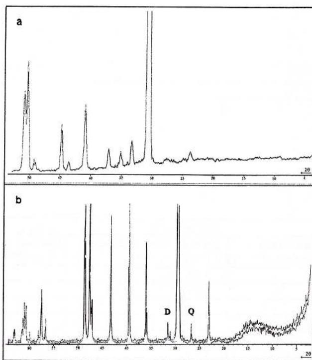
Fig. 2 - X-ray diagrams: a, dolomite; b, dolomite affected by dedolomitization (Q - quartz line; D - dolomite line; others are calcite lines).
