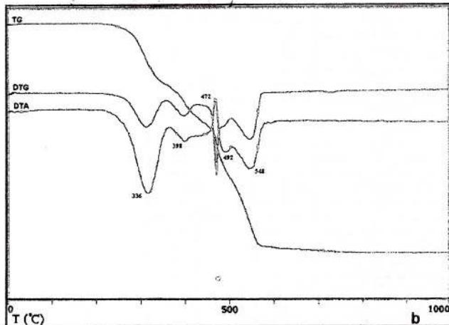
Fig. 4 – Thermal analysis of hydromagnesite (Valea Rea Cave)
