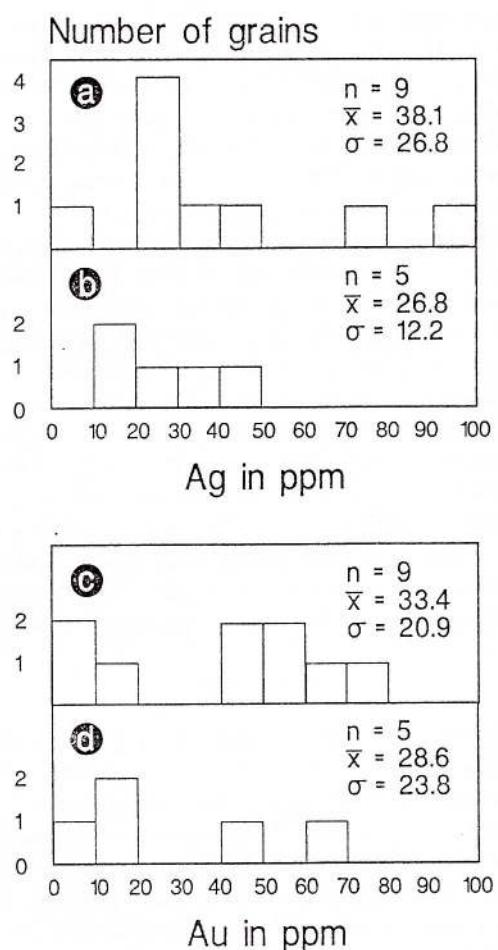
Fig. 7 - Histograms indicating concentrations of Ag in pyrite within (a) sample 22N (Nistru) and (b) sample 8255 (Herja) and Au in pyrite in (c) sample 22N (Nistru) and (d) sample 8255 (Herja).
