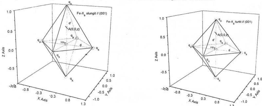
Fig. 6 - The elongated and shorted octahedron;  $|\Delta d| = 0.1d$
