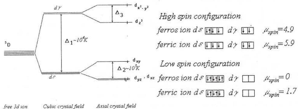
Fig. 1.5 - The ionic splitting of 3d shell in different symmetry of crystal field; and 3d spin configurations of iron ions
