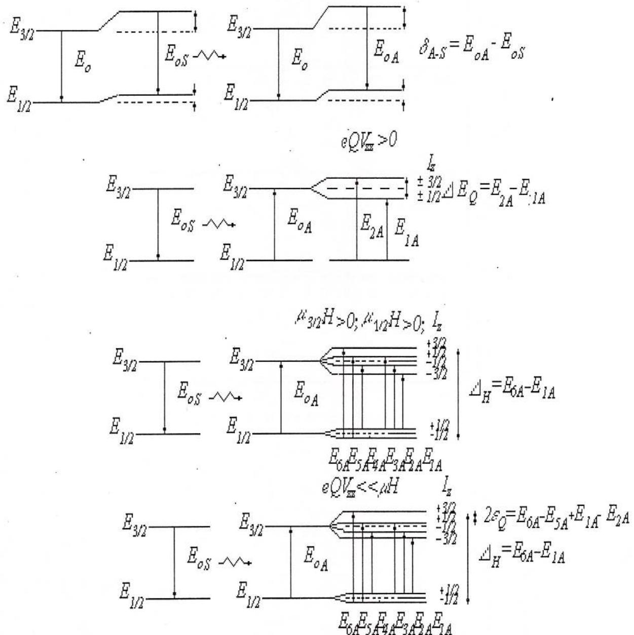
Fig. 1.6 - The splittings of nuclear levels in hyperfine fields
