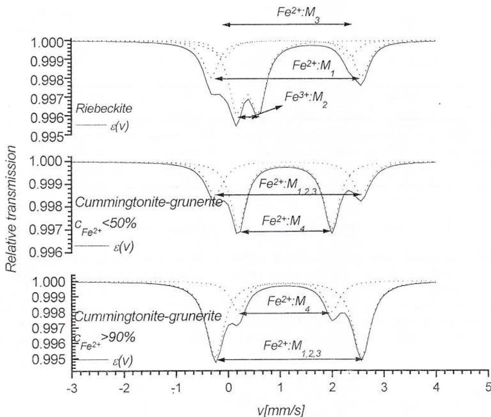
Fig. 2.5 - The iron sites in sodium and calcium amphiboles
