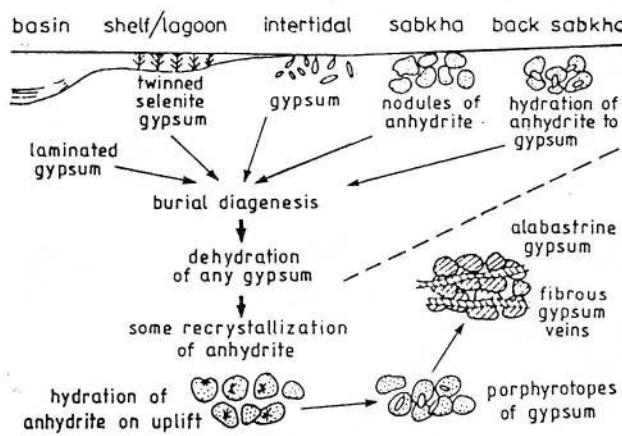
Fig. 6 – Genetic scheme for the sulfatic formations from the Meseş Area (after M. E. Tucker, 1991)
