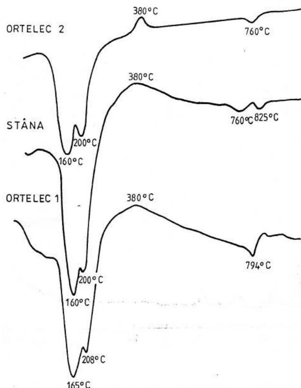
Fig. 2 - The DTA analyses of some gypsiferous samples
