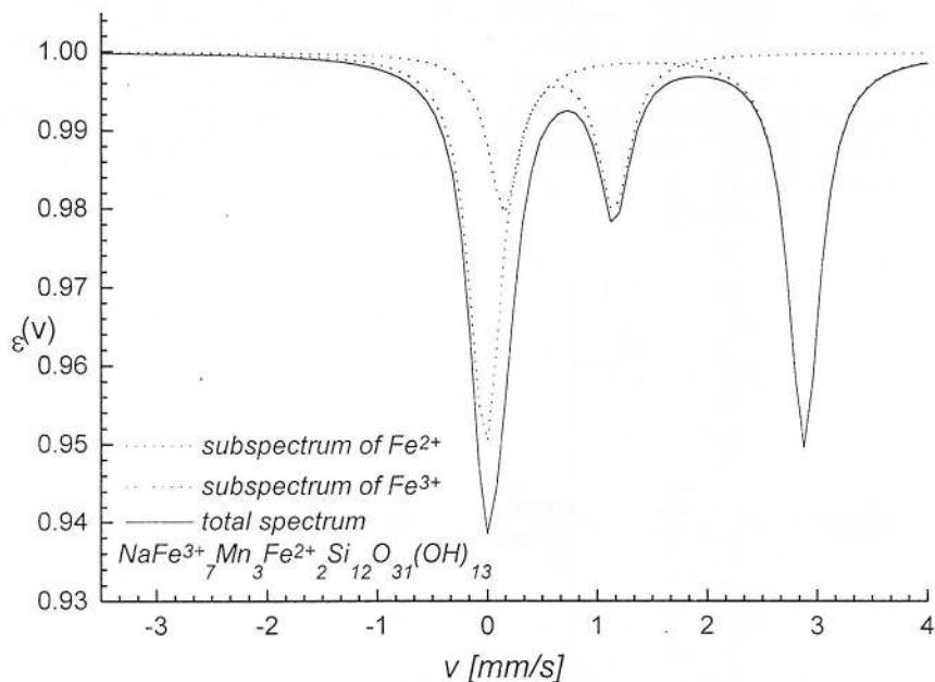
Fig. 2.2 - The Mössbauer spectrum of howite,  $\text{Na}(\text{Fe}^{2+}, \text{Mn})_{10}(\text{Fe}^{3+}, \text{Al})_2\text{Si}_{12}\text{O}_{31}(\text{OH})_{13}$ . (room temperature)
