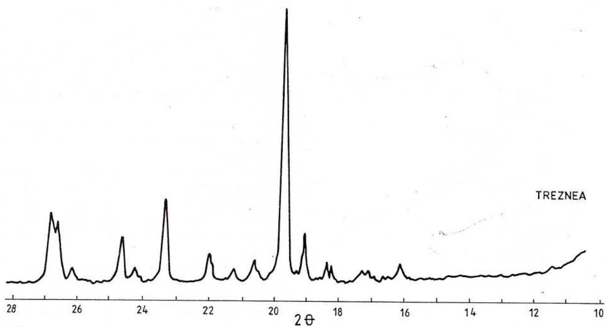
Fig. 4 – The X-ray analyses for the carbonatic impurities from gypsiferous samples (dolomite, calcite)
