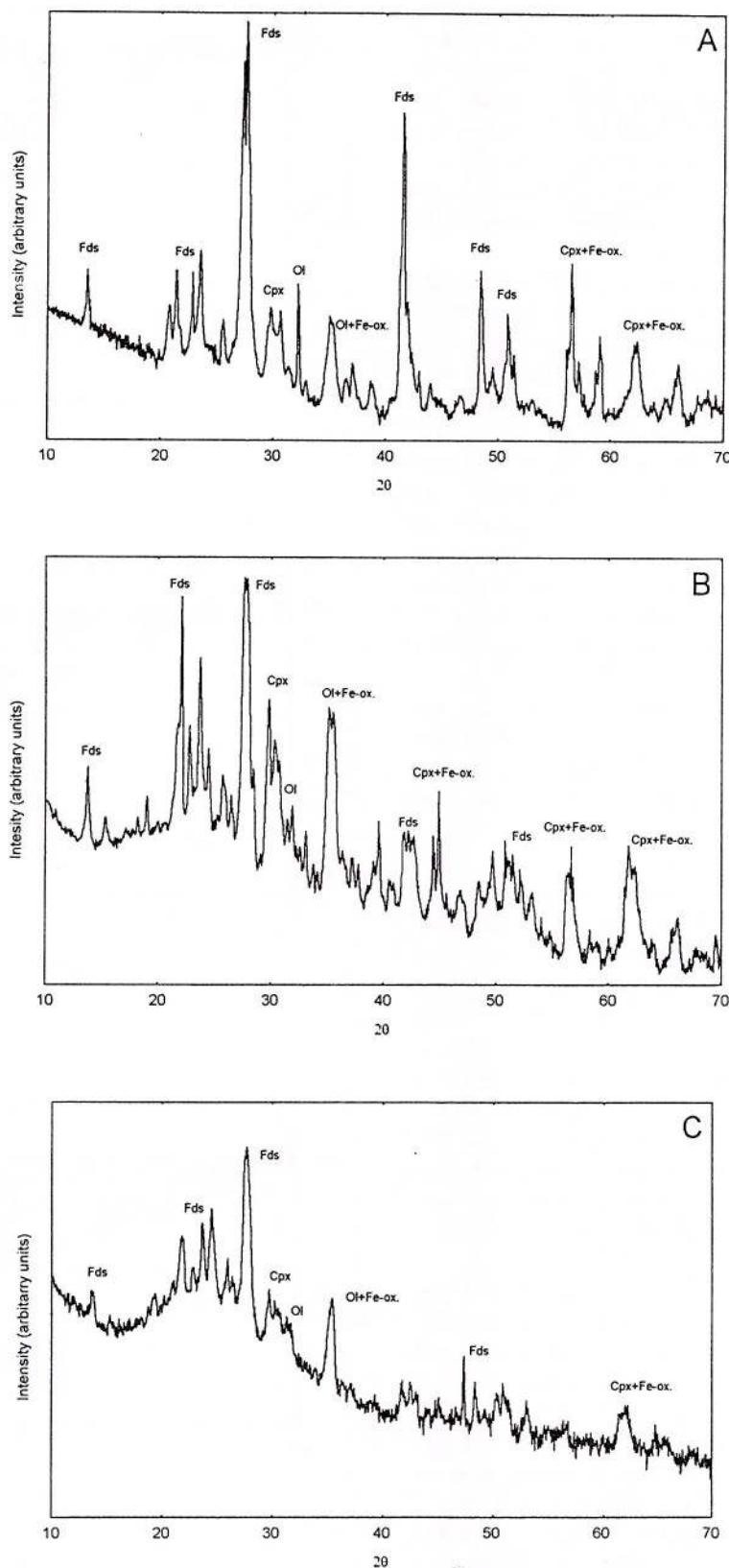
Fig. 2 - X-ray diffraction patterns for: A) the layer 0-2 cm of the marine soil; B) the layer 0-5 cm of the terrestrial soil; C) the layer 0-2 cm of the lacustrine soil. (Fds: alkali feldspar; Cpx: augitic clinopyroxene; Ol: olivine; Fe-ox: iron-oxides).
