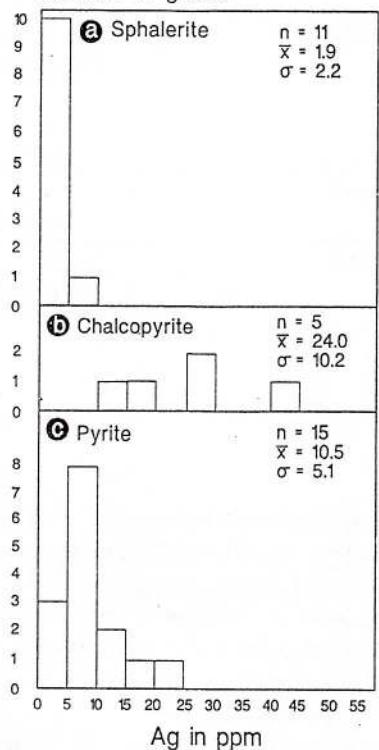
Fig. 3 - Histograms of Ag concentrations in (a) sphalerite, (b) chalcopyrite and (c) pyrite in the hydrothermal vein ores, expressed in ppm.
