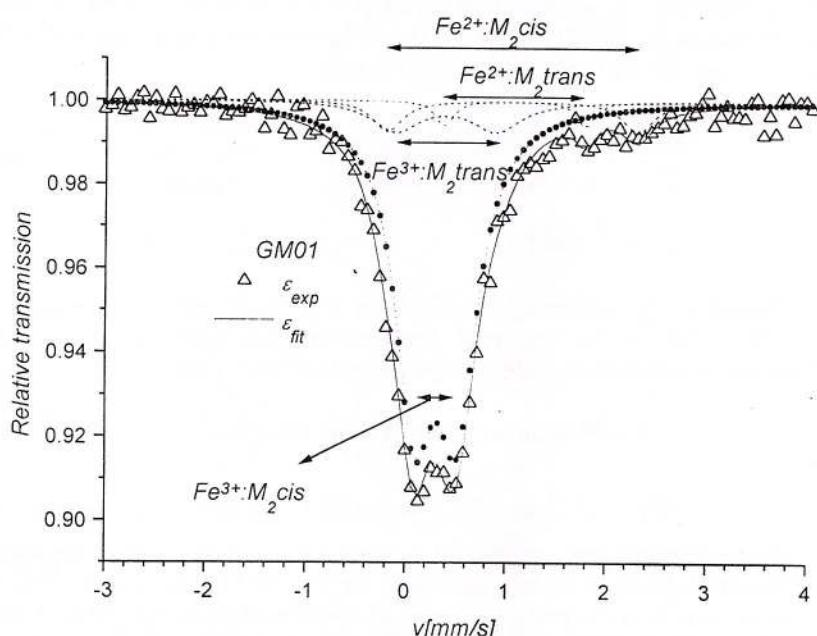
Fig. 3.3 - A typical Mössbauer spectrum of a glauconite
