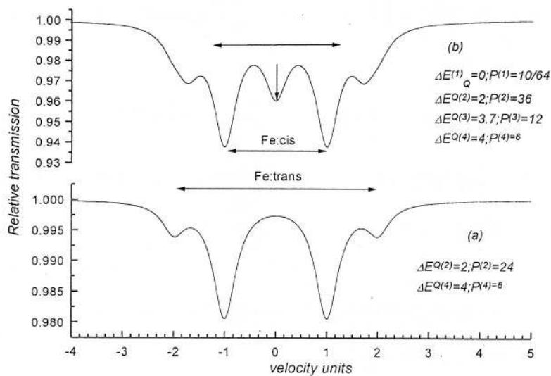
Fig. 2.10 - (a) Mössbauer spectrum of  $^{57}\text{Fe}$  in cis and trans octahedral sites; (b) Mössbauer spectrum of  $^{57}\text{Fe}$  surrounded by ionic  $(6-k)q_X^-$  and  $kq_Y^+$  charges.  $\Delta E_Q$  is given in  $eQ/8\pi\varepsilon_0$  units
