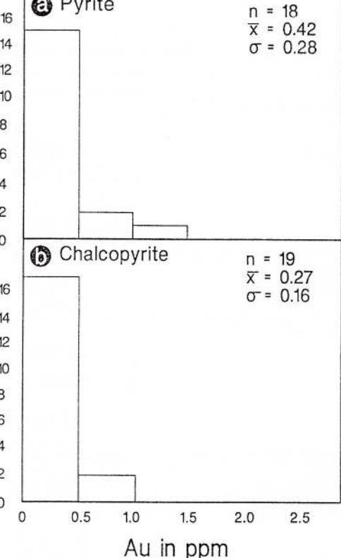
Fig. 2 - Histograms of Au concentrations in (a) pyrite and (b) chalcopyrite in the metamorphosed VMS ores, expressed in ppm.
