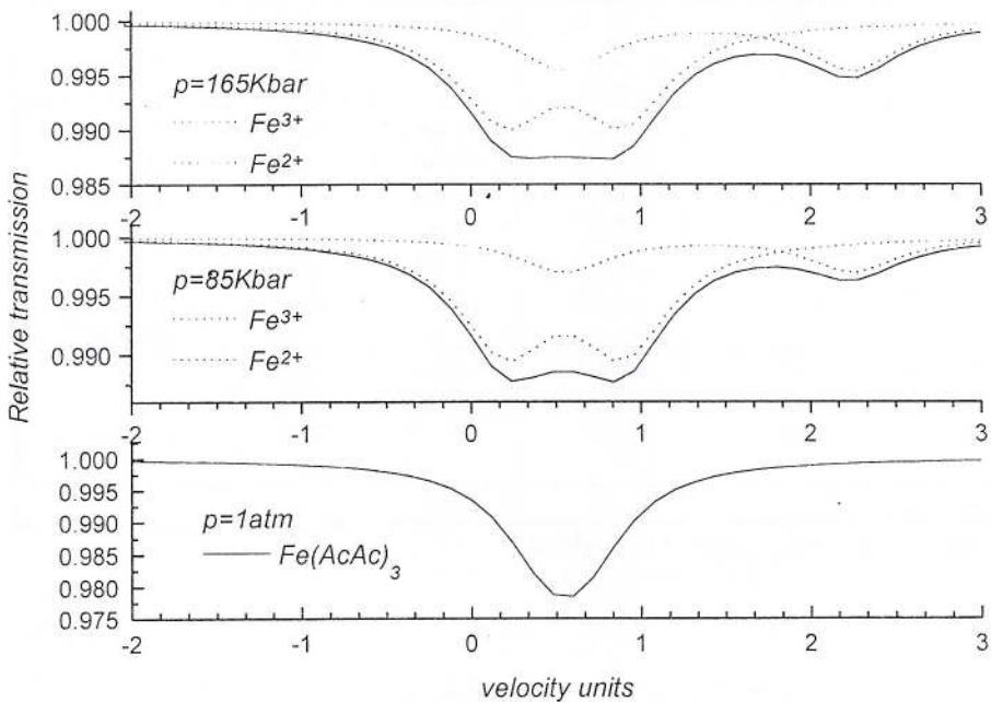
Fig. 2.13 - Mössbauer spectra of  $\text{Fe}(\text{AcAc})_3$  for different pressure conditions
