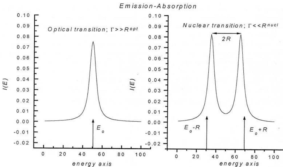
Fig. 1.2 - Emission-absorption processes for optical and nuclear transitions
