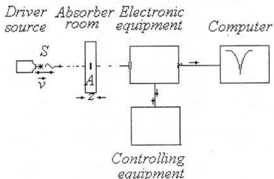
Fig. 1.4 - Basic Mössbauer equipment in transmission geometry
