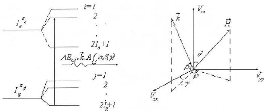
Fig. 2.15 - The splitting of Mössbauer isotope levels in coupled electric and magnetic hyperfine fields and the relative orientations of hyperfine magnetic field and  $\gamma$ -ray momentum to axes of EFG-tensor
