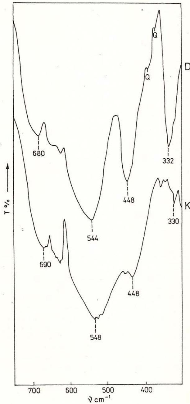
Fig.1- IR spectra of Kragerö ilmenite (K) and of Delinești pyrophanite (D).
