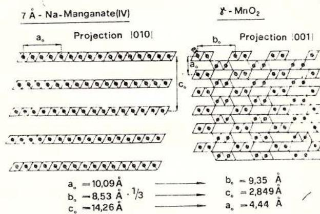
Fig. 4 - Schematic drawing illustrating the decay of the phyllo-manganate lattice to  $\gamma$ - $MnO_2$ . The  $\gamma$ - $MnO_2$  lattice is viewed along the needle axis.
