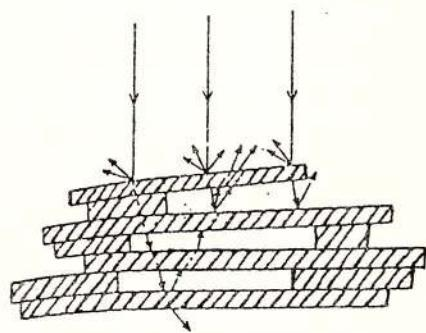
Fig. 7 - Schematic representation of a kaolin particle aggregate (Johns, 1986).
