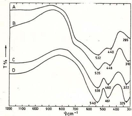
Fig.2- IR spectra for ilmenite of: A - Arendal, Norway; B - Kragerö, Norway; C - Chester, Vermont; D - Waterford - Rhode Island (Liese, 1967).
