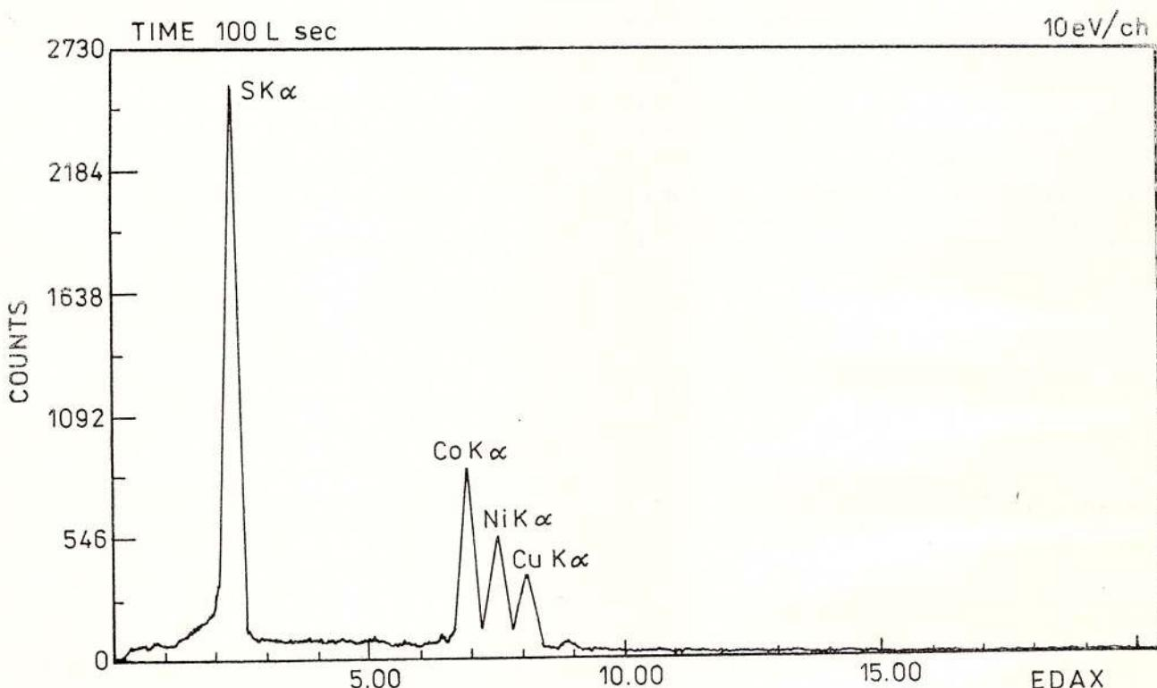
Fig. 2 - Characteristic energy spectra for fletcherite (?).
