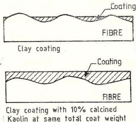
Fig. 9 - Function of calcined kaolin in paper coating (Clark, 1984).
