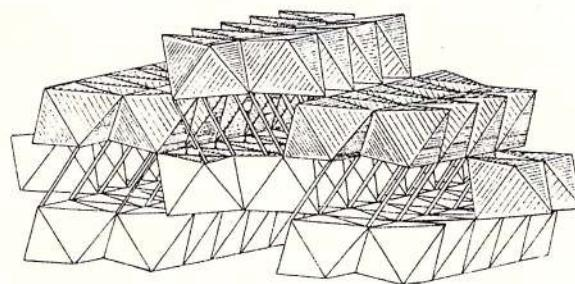
Fig. 5 - Goethite structure. The white diagonal sticks represent the hydrogen bond. These hydrogens can diffuse in and out of  $\gamma$ - $MnO_2$  as protons.
