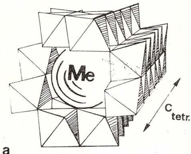
Fig. 6 - Schematic drawing of the structure of 2 x 2 tunnel manganates MeMn<sub>8</sub>O<sub>16</sub>. The size of Me is grossly exaggerated to underline the tight fit in the tunnel.
