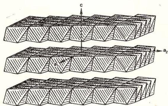
Fig. 1 - Schematic representation of the phyllophanate structure.  $[\text{MnO}_6]$  octahedra form the main layers by edge and corner sharing. The  $c_o$  distance depends on the interlayer content.
