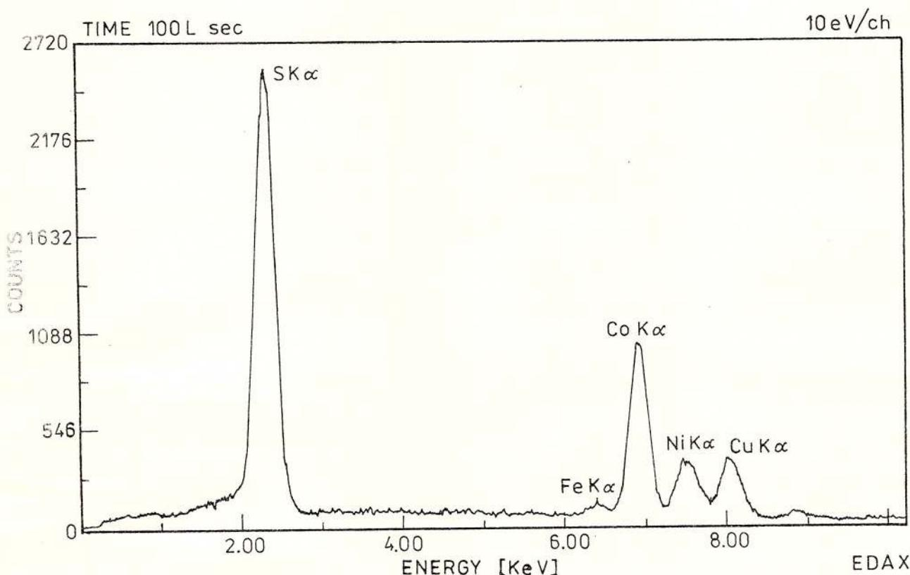
Fig. 1 - Characteristic energy spectra for carrollite.
