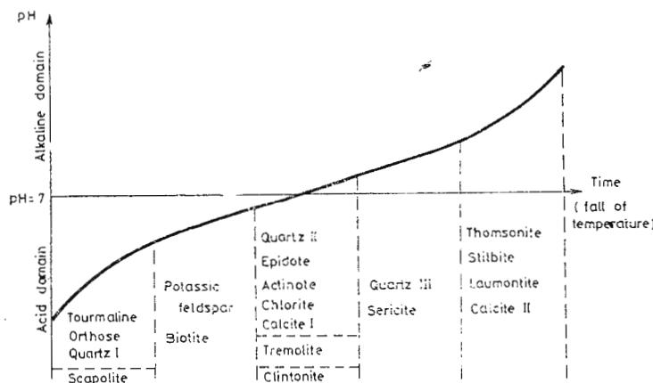
Fig. 3 — Evolution of the hydrothermal solutions pH.
