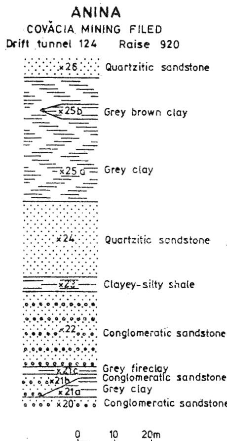
Fig. 2. — Stratigraphic column of the Lower Jurassic Fireclay Formation and location of samples in the Covăcia mining field.
