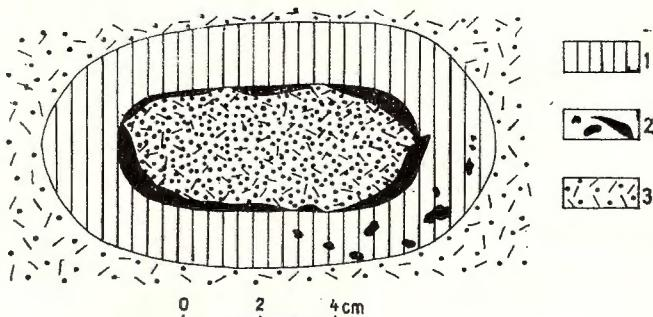
Fig. 1. — Section through a polymetallic ore lens.
