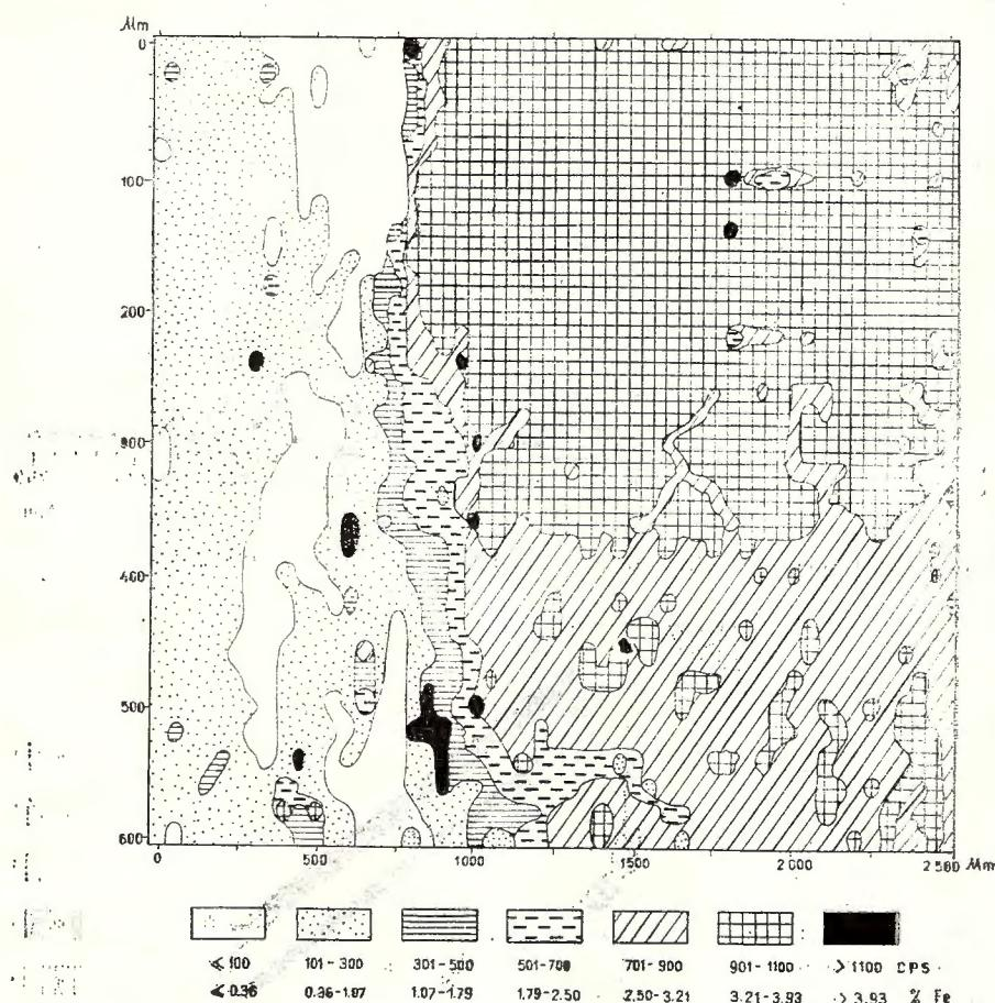
Fig. 10. — Counter map processed for areal distribution of iron within a single grain of sphalerite.
