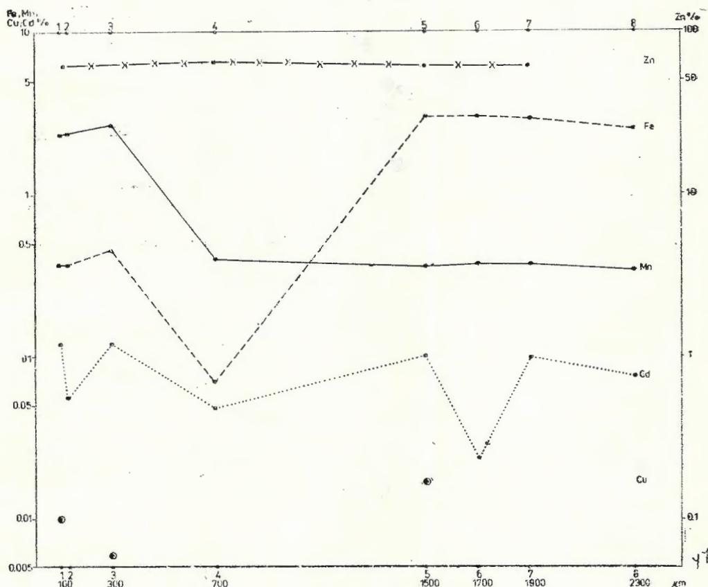
Fig. 5. — Variation diagram of Zn, Fe, Mn, Cd and Cu content within a sphalerite grain.
