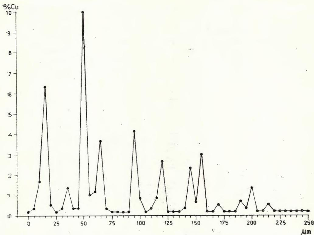
Fig. 8. — Linear distribution of copper within a sphalerite grain.
