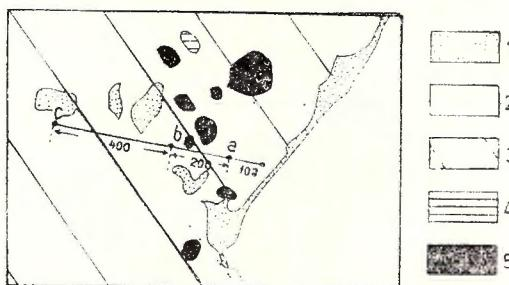
Fig. 4. — Location of microprobe traverse for the qualitative analysis on the polished section. 1, carbonates ; 2, galena ; 3, sphalerite ; 4, pyrite ; 5, vugs ; a, b, c, qualitative point analyses ; 100, 200, 400-distance in  $\mu\text{m}$ . For general setting see plate I, fig. 1.
