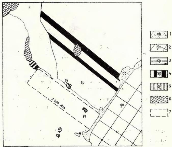
Fig. 9. — Position of counter map on the polished section. Grain boundaries developed by etching. 1, carbonates; 2, galena; 3, chalcopyrite; 4, sphalerite with twinning lamellae; 5, pyrite; 6, vugs; 7, map outline.
