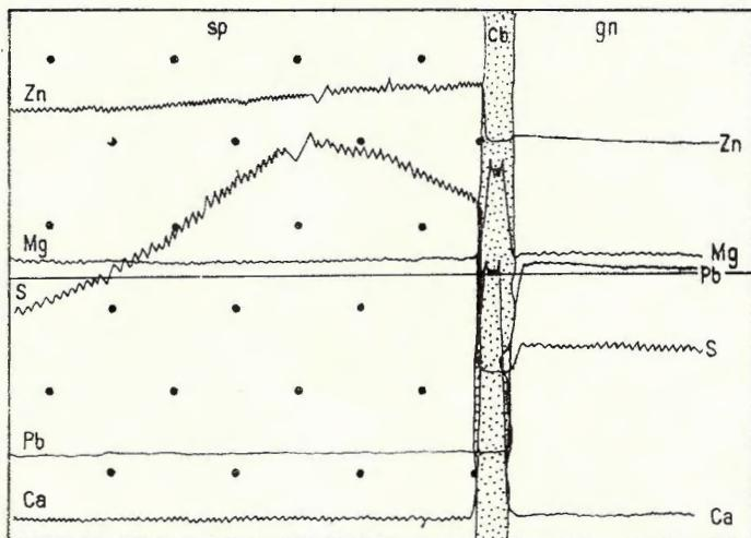
Fig. 3. — Line scans of the elements  $ZnK_{\alpha}$ ,  $PbL_{\alpha}$ ,  $SK_{\alpha}$ ,  $CaK_{\alpha}$ , and  $MgK_{\alpha}$  at the boundary between sphalerite (sp) and galena (gn), where there is a narrow band of carbonates (cb).
