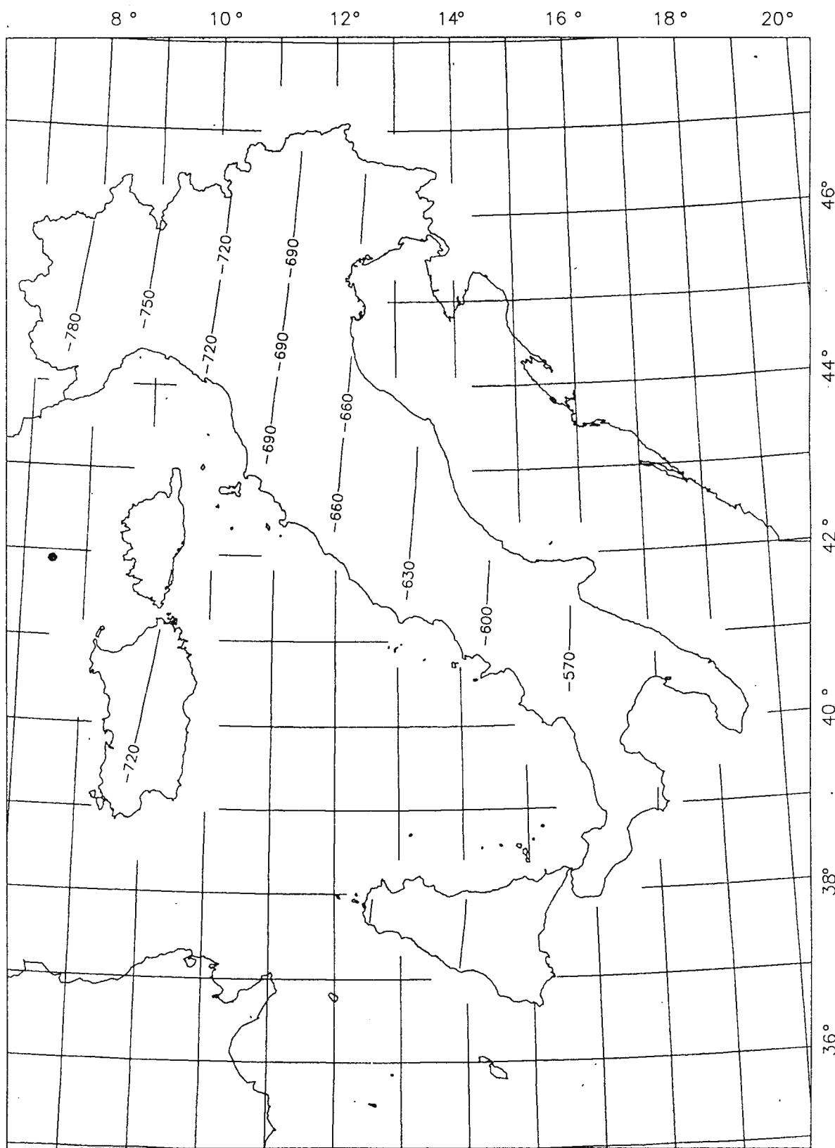
Fig. 6 – Contour map of declination reduced at 1890.0 using normal field approximation
