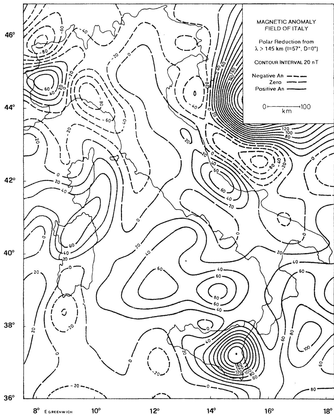
Fig. 4 – Polar reduction from low-pass filtered map ( $\lambda > 145$  km) of magnetic anomaly field of Italy.
