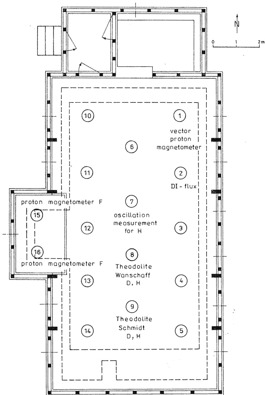
Fig. 2 - Lay-out of the instruments in the absolute house
