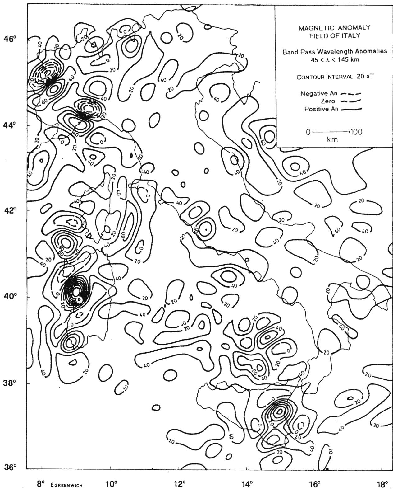
Fig. 3 – Band-pass filtered map of magnetic anomaly field of Italy ( $45 < \lambda < 145$  km)
