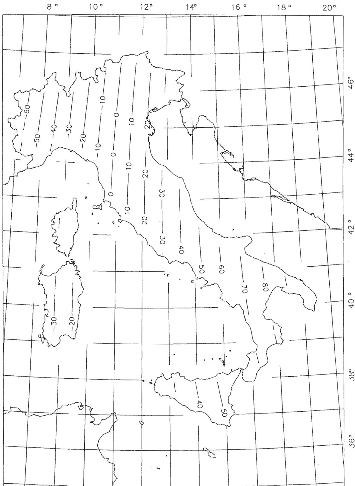
Fig. 7 – Contour map of declination reduced at 1990.0 using normal field approximation
