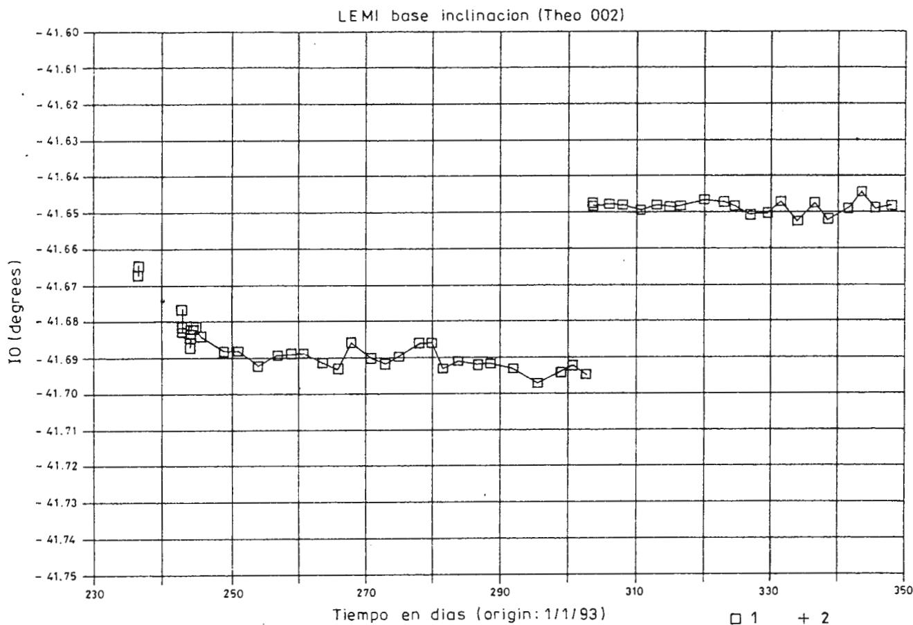
Fig. 4 – Evolution of the inclination baseline of the variometer as given by the DIflux for more than 100 days after the installation in Trelew. The jump on day 303 is due to a baseline adjustment.
