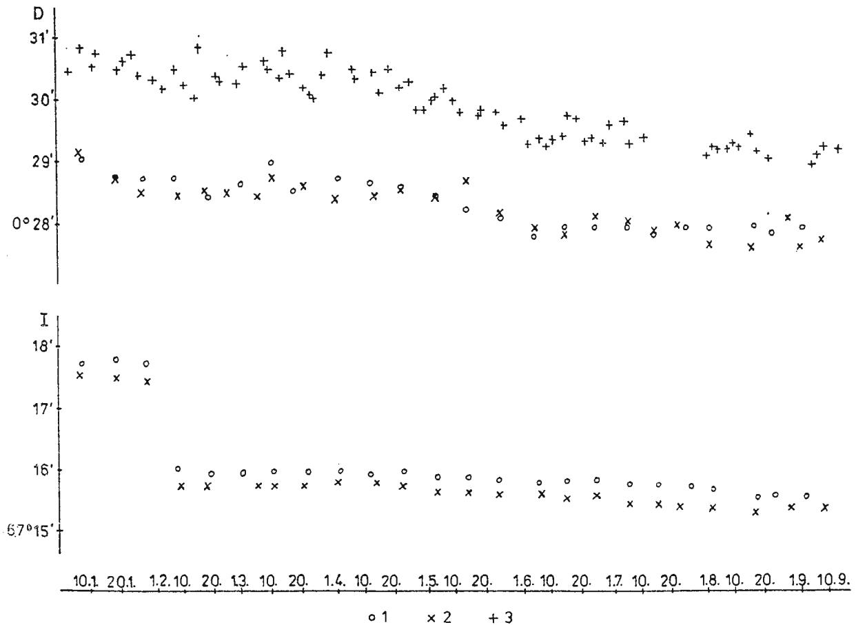
Fig. 3 – First results of the comparison of absolute measurements of D and I at Niemegk observatory in 1992. o, classical method; x, DI-flux; +, proton vector magnetometer.
