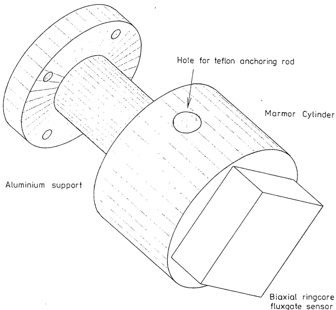
Fig. 2 – The aluminium-Teflon-marmor assembly. It allows the mounting of the biaxial fluxgate on an inclinometer frame. It is held by 4 screws at the rear. The hole in the marmor cylinder allows insertion of a Teflon rod on which the fluxgate is fixed by two screws (not shown). An axial screw in the aluminium support also clamps the marmor cylinder on the support by insertion in the Teflon rod.
