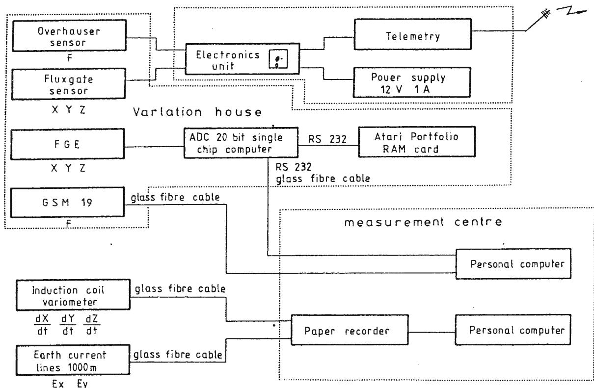
Fig. 1 – Conception of new recording systems at Niemegk Observatory
