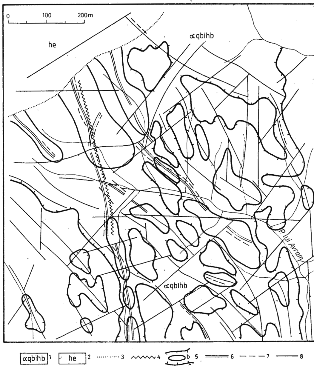
Fig. 3 - Structural and metallogenetic sketch-map of the Piriul lui Avram zone inferred from \Delta T magnetic and gamma-ray spectrometric data.
