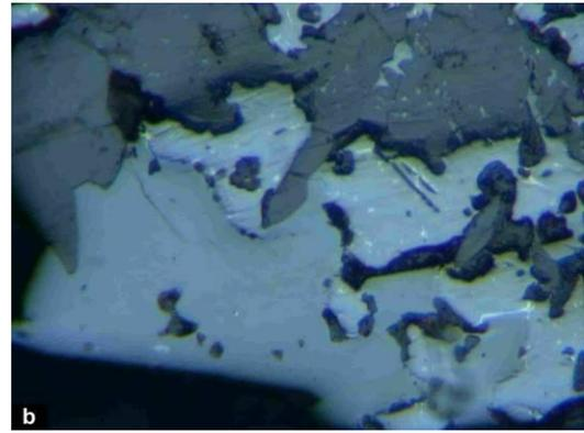
Figure 1. (a) Native iron (white, blebs) in wüstite (grey white); (b) wüstite (grey), magnetite with troilite inclusions (whitish grey) and fayalite (dark grey) with wüstite inclusions. Reflected light, x160, NII.
