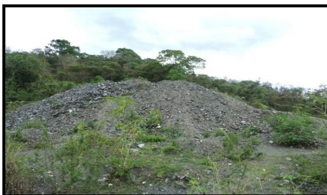
Fig. 2. Example of waste material used in the experiments. The material is composed of different schists, amphibolite and quartz veins.
