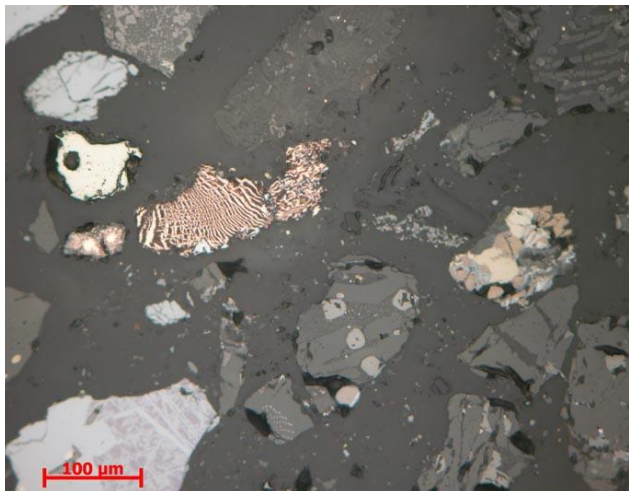
Fig. 5. Chalcocite, bornite, chalcopyrite, copper containing interdendritic cuprite, glass with magnetite. NII, reflected light.
