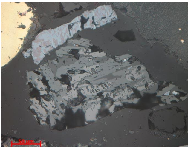
Fig. 13. Prismatic fayalite and magnetite in glass, copper drops. NII, reflected light.
